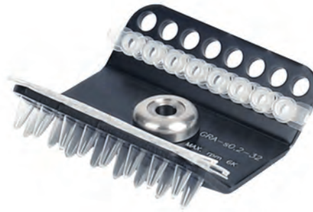
PCR Rotor - CODE 1042 32 x 0.2 ml Tubes 13500 RPM / 12300 X g
